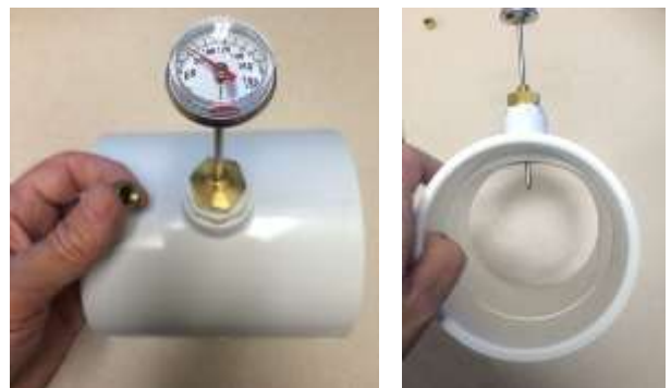
Probe inserted into port when measuring water temperature to and from the heat pump
