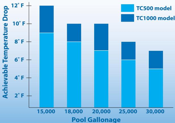
Extreme climates with consistent temperatures in excess of 100° F may experience the need for extended runtimes, larger units or multiple units.
