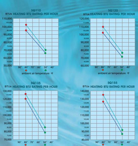
ambient air temperature °F ambient air temperature °F 63% RELATIVE HUMIDITY / 80° WATER TEMPERATURE - RATED IN ACCORDANCE WITH ARI STANDARD 1160 80% RELATIVE HUMIDITY / 80° WATER TEMPERATURE - OUTSIDE THE SCOPE OF ARI STANDARD 1160 HIGH TEST POINT TEMPERATURE • LOW TEST POINT TEMPERATURE
