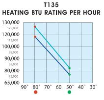
80% RELATIVE HUMIDITY / 80° WATER TEMPERATURE 63% RELATIVE HUMIDITY / 80° WATER TEMPERATURE \*
